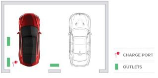
Install near vehicle charge port, maximum 15' away, minimum 18" above ground
